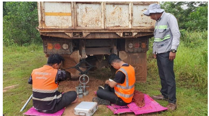
Fig. 3. In-situ CBR testing at the site
